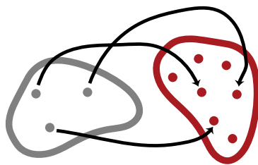
Figure fun.3: An injective function never maps two different arguments to the same value.
